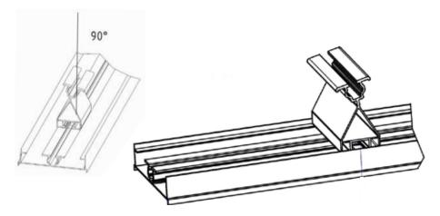
Observe the appropriate module and row distances for the profile and module installation.
