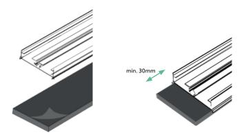
The installation distances of the structural protection mats below the base profile depend on the selected installation version.
